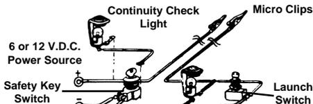
This circuit includes a continuity check light. This is a small bulb (no more than 1/4 amp for safety) that lights when a complete circuit exists between battery and igniter; this indicates that the rocket can be launched. If the continuity check bulb does not light when the safety interlock is closed, check to see if the micro-clips are properly connected to the igniter (always remove the safety key before checking the igniter!).
