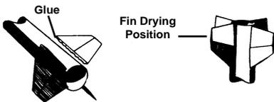
Sometime after the fin joints have dried completely, they should be reinforced. Do this by applying a "fillet" of glue as shown. Always support the body in a horizontal position while fillets are drying so that the glue does not run. Build up the fillets in several thin layers, allowing each layer to dry between applications (this is much faster than waiting for a single thick fillet layer to dry).
