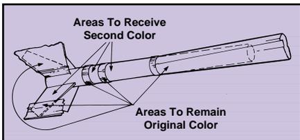
With the model masked, apply an additional thin coat of the first color to finish sealing the edges of the tape. When this is dry, apply the second color in several thin coats. Use just enough paint to get good color. After the last coat is dry, remove the masking carefully to avoid peeling the paint. A third color would be applied in the same way as the second.
