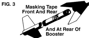
After taping the engines together, wrap masking tape around the upper stage engine at the front and near the rear as in figure 3 to give it a tight fit in the body. Push it into place. Wrap the booster engine and push it into position. Failure to get the upper stage engine in place tightly enough will result in the recovery system malfunctioning; failure to secure the booster stage tightly can result in its dropping off under acceleration.
