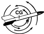
The most significant forces acting on a model rocket in flight are caused by the thrust of the engine, the action of air on the nose and the action of air on the fins. Off-center thrust and forces on the nose try to bring the nose of the rocket around to the rear. They are opposed by the forces acting on the fins. All these forces are amplified by the distance from the location of the force to the center of gravity.
