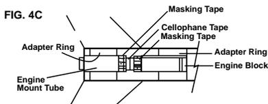
In some multi-stage models the engines cannot be coupled directly together with cellophane tape, such as the case where a D12 is staged to a standard size engine. In this case, use masking tape on the stage couplers as needed to achieve a tight fit between stages, to prevent separation before upper stage ignition.
