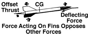
As long as the forces on the fins of the rocket are great enough to counteract the forces on the nose and any off-center thrust, the rocket will fly straight. If the fins are too small and/or too close to the center of gravity, there will not be enough force to counteract the force on the nose. As a result, the nose will swing out to the side and the model will try to chase itself around the sky.
