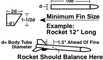
The third rule is to place the fins as far back on the rocket as possible. Generally, this means that the rear edge of the fin will meet the rear end of the body and the fin will be swept back. Do not place any fins ahead of the center of gravity!
