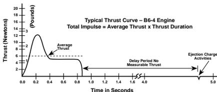
The combustion of the solid propellant produces high temperature, high pressure gases that are ejected through the nozzle. The reaction to forcing the exhaust out the nozzle is a forward thrust (an example of Newton's Third Law of Motion). During the thrust phase the model rocket accelerates upward, gaining velocity and altitude.
