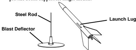
The blast deflector is a metal plate that prevents the engine exhaust from hitting the launch pad or ground, preventing fires. Heavier rockets will require thicker launch rods and a launcher with a heavier base. Bricks or rocks can be used to weight the base when extra-large models are being launched.
