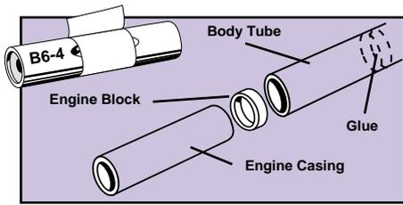
When mounting the engine in a model with an engine block, wrap the engine with masking tape until it makes a tight friction fit in the tube, then slide the engine into place. If the fit is too loose, the engine will kick out at ejection and may not deploy the recovery system. If the fit is too tight, you may damage the model trying to push the engine in place. Adjust the amount of tape as needed.
